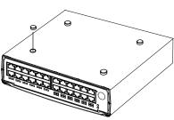
a. Set the device on a flat surface near an AC power source, making sure there are at least two inches of space on all sides for proper air flow.
